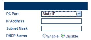
Enable the DHCP Server if you want the GoIP\_4 Gateway functions as a local DHCP host for the PC segment. This will enables the GoIP\_4 Gateway to assign IP Addresses to network devices that are attached to the PC port segment.
