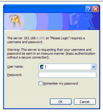
Enter the User name and Password and the press OK to access the GoIP\_4 Gateway Web Server. The default for both user name and password is "admin".
