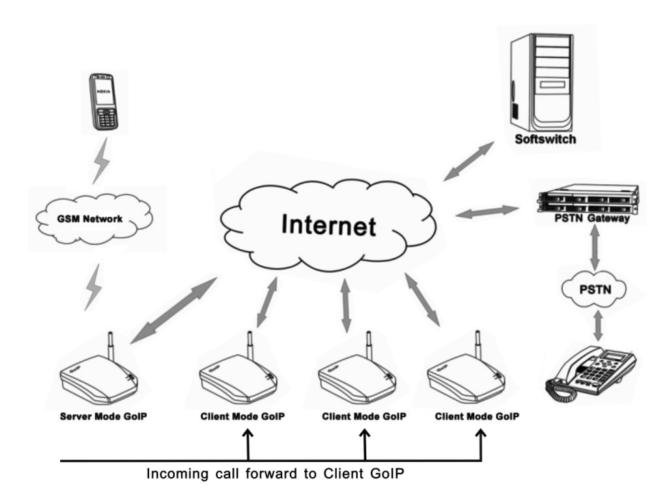
GoIP\_4 supported multi\_devices cooperate with one group; it can work like a multi\_channels GSM gateway. Any one GoIP\_4's channels are can work as **Group Server Mode** or **Client Mode**.
