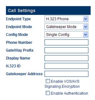
The "Gatekeeper Mode" mode allows a user to setup the GoIP\_4 Gateway by registering to the gatekeeper with one H.323 account.
