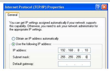
Set an unused IP address that is in the same segment as the PC port address.
