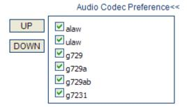
Click on the check box to enable a codec. Select a codec and then press the UP or DOWN button to move the position of the codec on the codec list with a priority in descending order.
